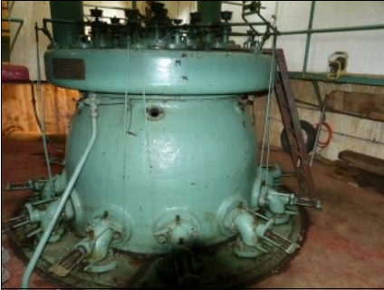
Ignition chamber of the Humphrey Pump.
