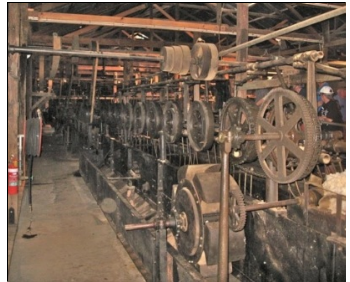
An operating scour line in 2009
