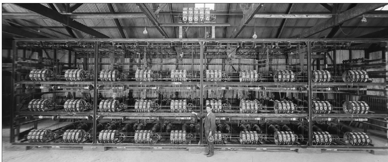
Front view of the first 1913 Tote, assembled for testing in Sydney before shipping to NZ. Photo courtesy the Powerhouse Museum, Sydney.
