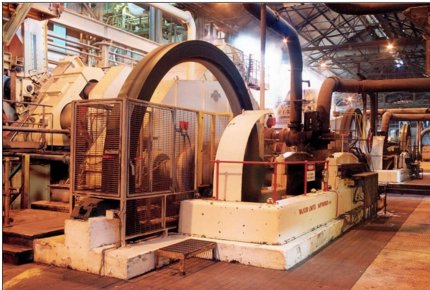
The Millaquin sugar cane crushing mill, made by Walkers Ltd, Maryborough, Qld. Photographed while it was still working in Bundaberg. Photo: Bundaberg Sugar
